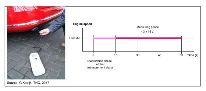
The particulate measurement can be performed regardless of the operating state (cold/warm, EGR valve open/closed) of the engine since a diesel engine with a faultless filter usually emits significantly less than 3'000 1/cm<sup>3</sup> at low idle, i.e. much less than what is set as the limit for passing the test (see section 5). There is therefore no need to condition the engine before the test procedure.
