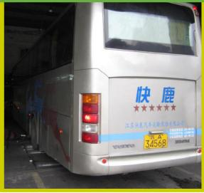
One of the busses used in the Xia Men project for real driving emission and chassis dynamometer measurements
