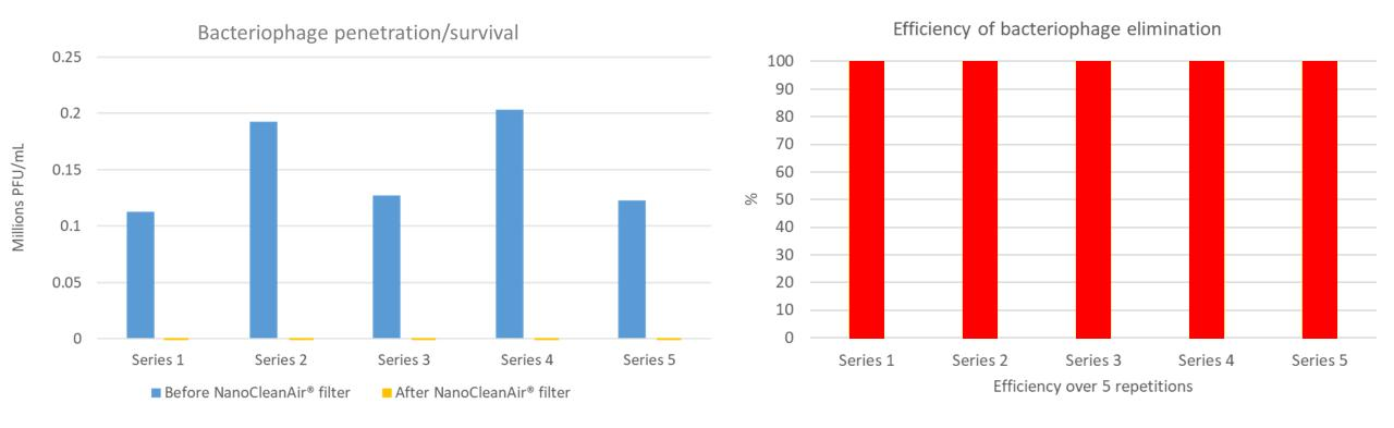
The efficiency of virus (bacteriophage) elimination by NanoCleanAir® filter is > 99% (n=5)
