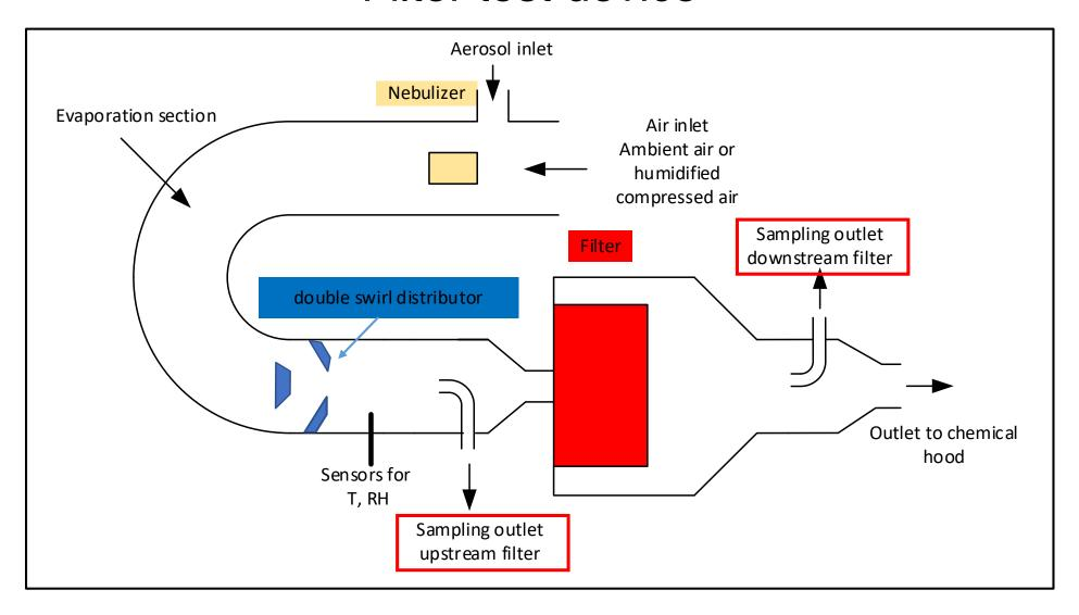
T= 21°C; RH = 40–50%; flow rate  $\approx$  20 m<sup>3</sup> h<sup>-1</sup> main flow and 5 L min<sup>-1</sup> sample flow
